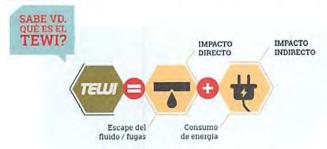
The installations made with RS-50 (R442A) are installations for the future that can be maintained without ban dates thanks to the GWP of 1888. Being a low GWP solution, in case of leakage, we will reduce direct CO<sub>2</sub> emissions (direct impact).
